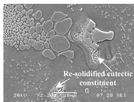
Figure 3 Melting of terminal solidification constituents at 1155 °C.
