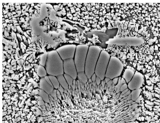
Figure 1 SEM secondary electron image showing eutecticlike constituent ahead of  $\gamma$ - $\gamma'$  eutectic.
