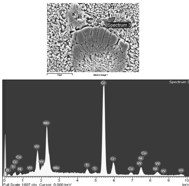
Figure 4 EDX spectrum from Cr-Mo boride.
