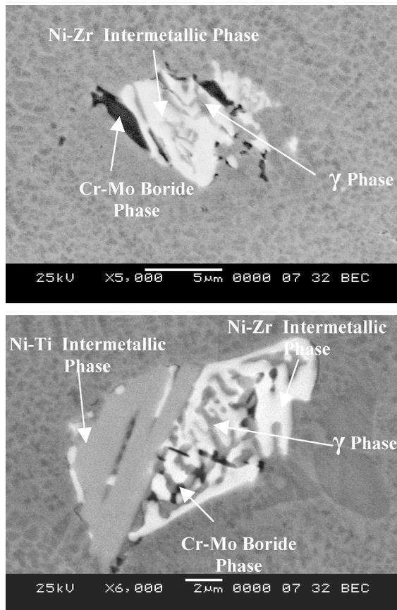
Figure 2 (a) SEM backscatter electron image of ternary eutectic-like constituent. (b) SEM backscatter electron image of quaternary eutectic-like constituent.
